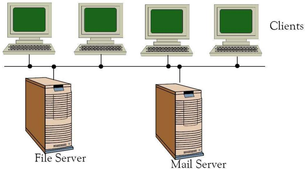
Figure 1.12. Typical server-based network architecture
